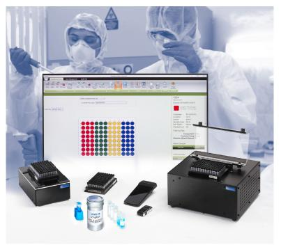
of Ziath's Samples software, the rack scanner and picker can work seamlessly to provide verification of original tube position in a rack and the location of any picked tube in a daughter or destination rack, updating the database with both pieces of information in real time.
